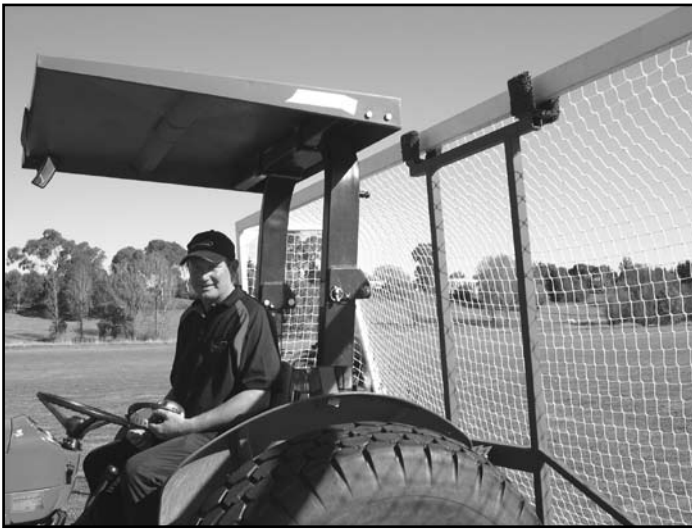
The cost-and-injury-saving “Goal Shifter” was the brainchild of UNE Grounds Assistant Terry Farrell and OHS Officer Graham Bruce. Previously, it took at least three people to handle the heavy steel soccer goals manually; the new invention, using a tractor’s three-point linkage, makes it a one-man job. The invention was a finalist in the WorkCover NSW OHS Safety Award.
