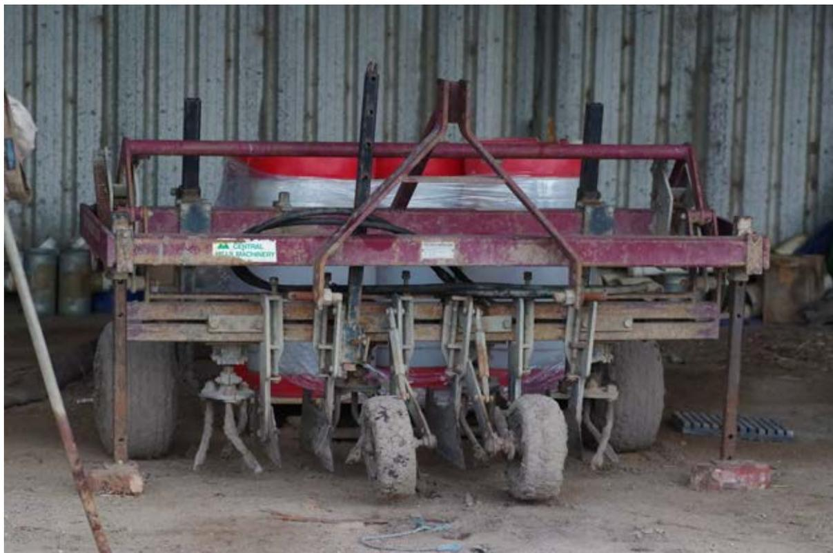
Figure 2. A Weedfix inter-row cultivator similar to the one used on the Victorian Case 3 farm
