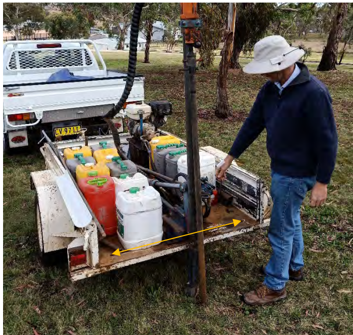
Figure 5 (The soil sampler can be positioned to the left or right side of the trailer by pushing it along the track built into the floor.)
