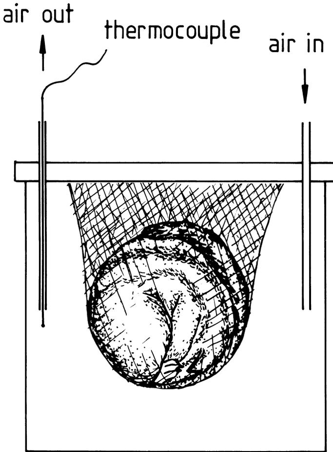
Fig. 1. Experimental setup for cooling experiments. Animals were suspended in a plastic mesh hammock in the respirometer to maximize heat exchange with surrounding air.
